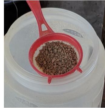
Image 3: Dried clay was pulverized into a powder
