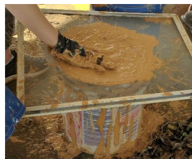
Image 1: Slip was screened through a 18x16 mesh
