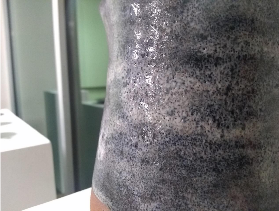
Image 7: Significant pinholing was observed in glaze for clay #3
