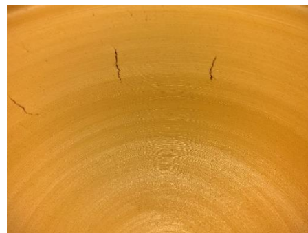
Image 5: Stress cracks developed during throwing a large bowl
